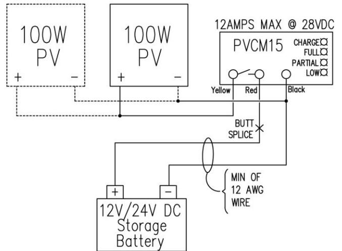
Before mounting the PVCM15 regulator inside the solar panel junction box, clean the surface to which the PVCM15 will be attached. Allow the surface to dry. Remove the backing from the double stick tape and press firmly into box cover.
