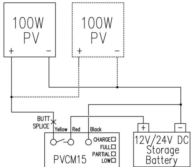
Connect the PVCM15's regulator wires to battery terminals and attach regulator to battery cables with a tie-wrap.
